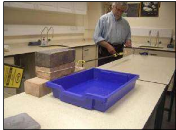
Brickquake, pulled by a winding mechanism (ESEU)
