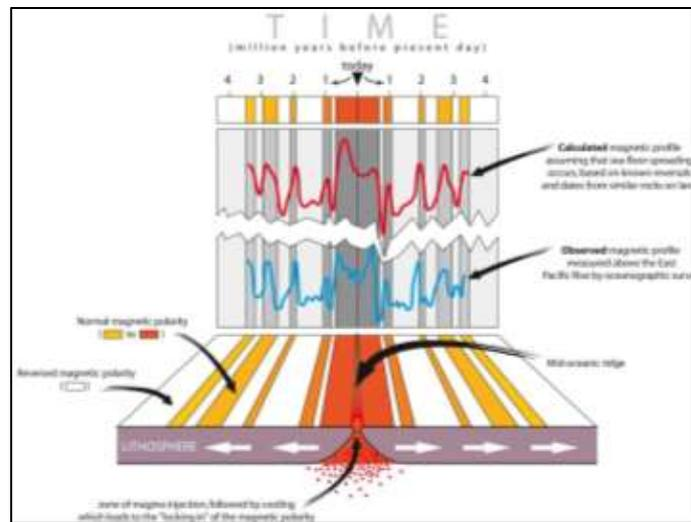
Magnetic evidence for ocean floor spreading
