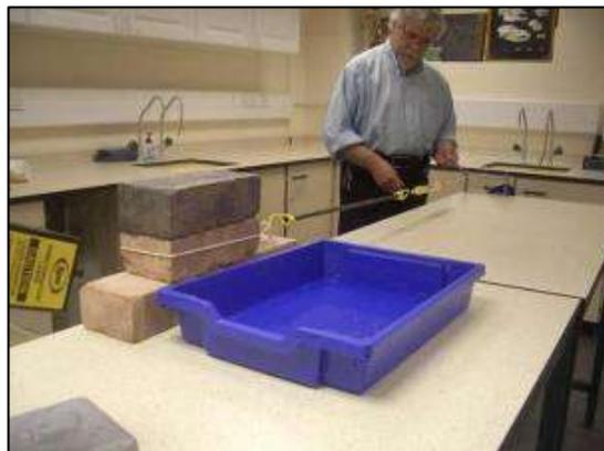
Brickquake, pulled by a winding mechanism (ESEU)
