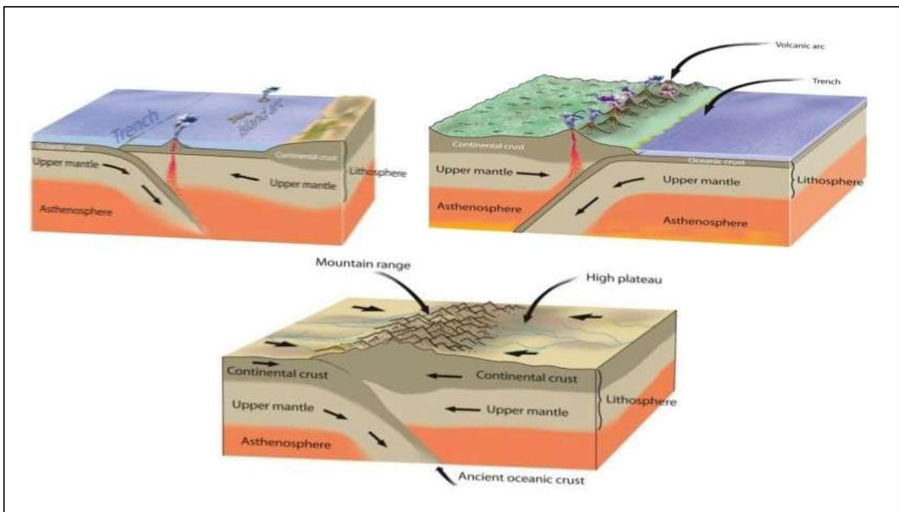
The three types of destructive plate margin, reproduced with the kind permission of the US Geological Survey, redrawn by ESEU.
