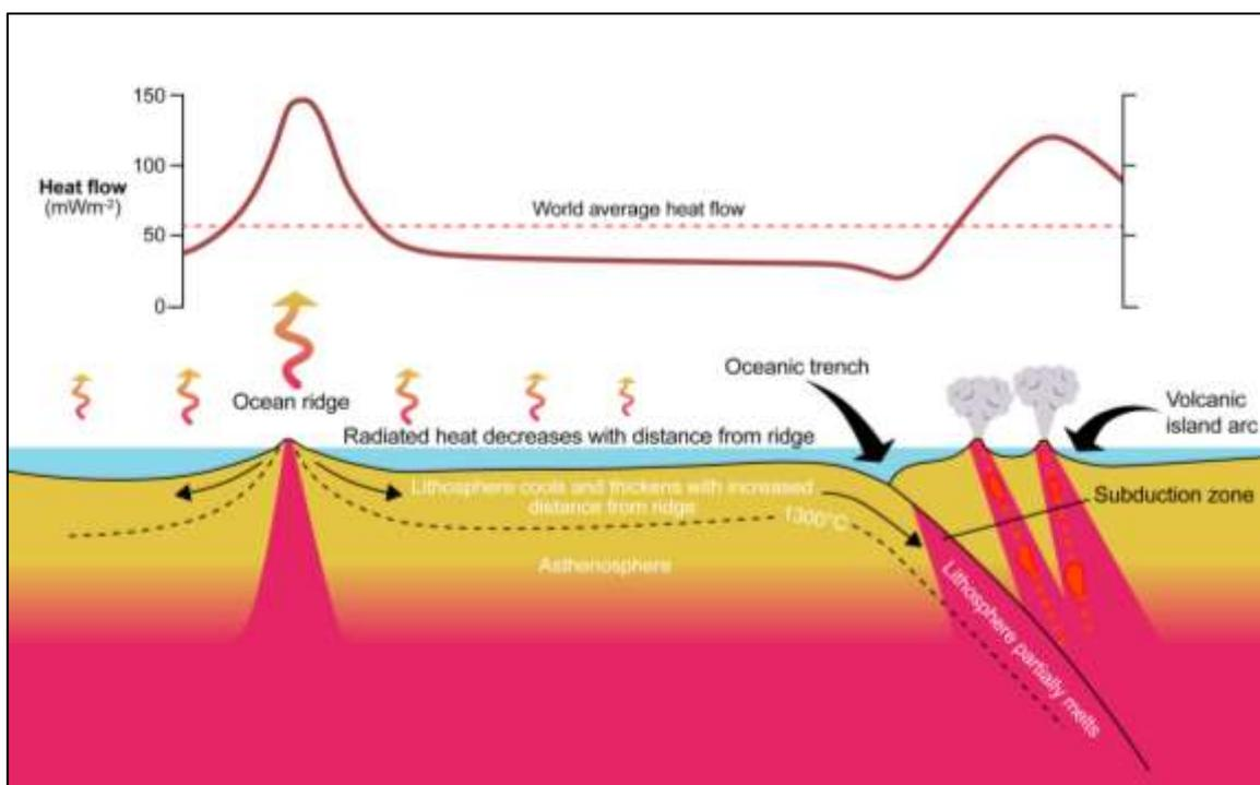
The pattern of heat flow out of the ocean floor and the upper part of the mantle and the crust.
