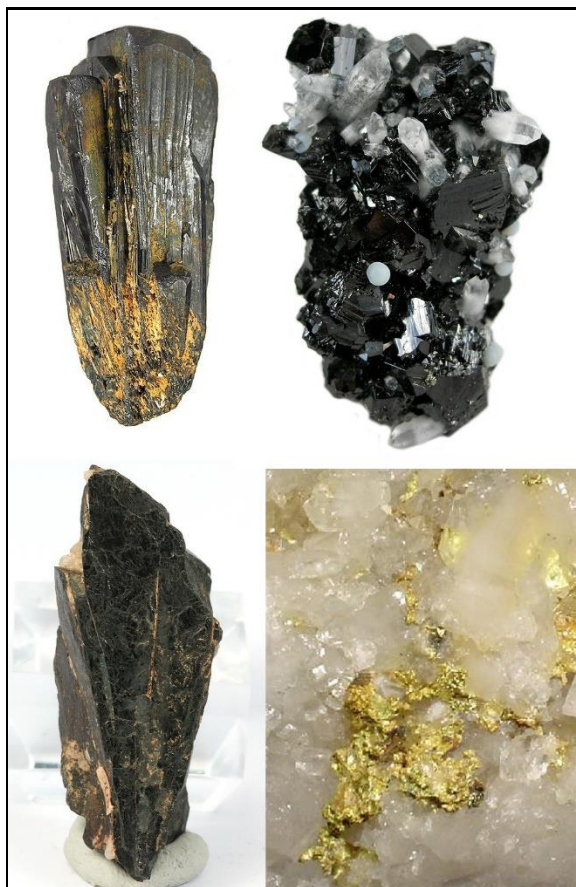
Fig 1. Ores of the “Three Ts” and gold: clockwise from top left: coltan (Ta and Nb); cassiterite (Sn), gold (Au) and wolframite (W) (This file is licensed under the Creative Commons Attribution-Share Alike 3.0 Unported license. Attribution: Rob Lavinsky, iRocks.com – CC-BY-SA-3.0)
