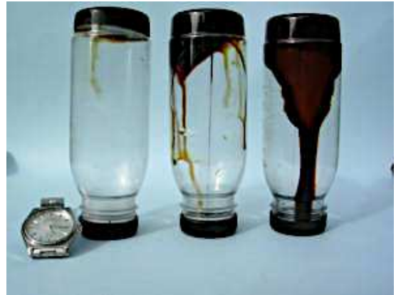
Fig 1 Treacle at three different temperatures, where the containers have been inverted at the same time (Photo P. Kennett)
