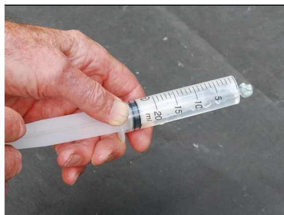
Water in the syringe beginning to boil and to produce bubbles of water vapour as the pressure is reduced by pulling back the plunger.
