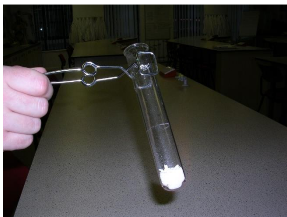
Heating ground gypsum in a Pyrex™ boiling tube, with water droplets condensing near the top of the tube. (The Bunsen flame is invisible in this photograph). (Photo: P. Kennett)
