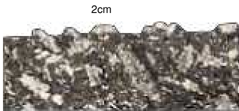
Detail of crystal wear in a rock fragment
