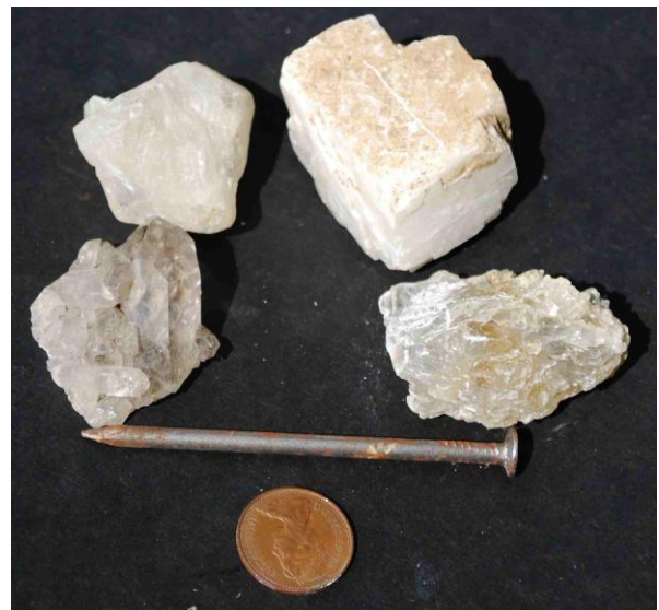
4. Hardness: fluorite, calcite, gypsum, quartz, with a steel nail and a 'copper' coin
