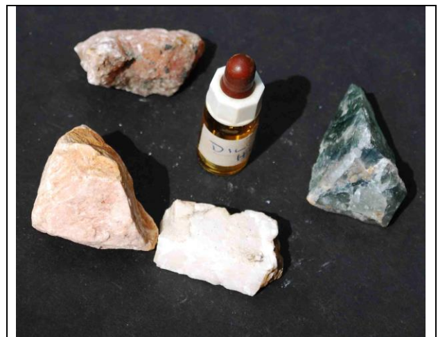
5. Acid test: gypsum, fluorite, calcite, barite and a dropper bottle of dilute hydrochloric acid (All photos: Peter Kennett)
